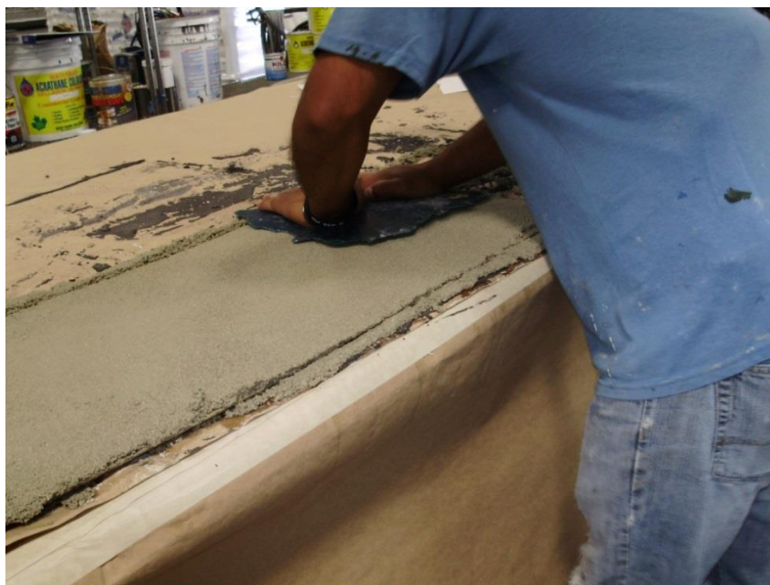
Figure 2-11 Testing Fluoropolymer Coating on Stamp Mat
