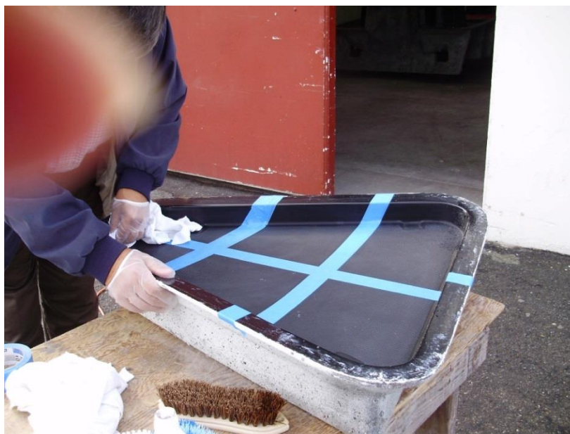
Figure 3-2 Cleaning Test of PCBTF at Boat Manufacturer
