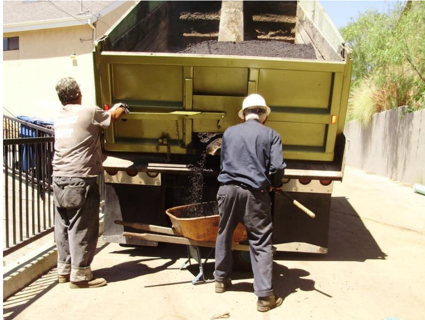
Figure 2-23 Release Agent Testing on Truck Liftgate
