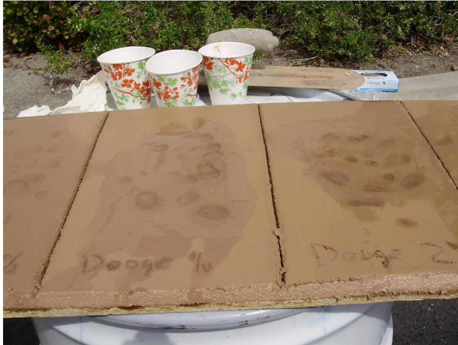
Figure 2-6 Preliminary Stamping Tests with Dodge Oil Release Agent
