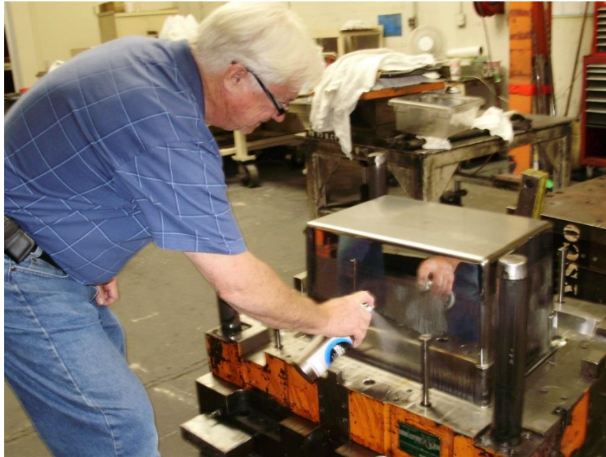
Figure 3-16 Spraying Baseline Hexane Aerosol on Mold
