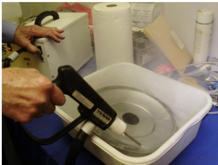
Figure 3-17 Testing Alternative Cleaner on Metal Mold
