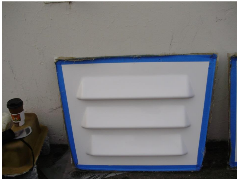
Figure 3-4 Part Made with PTBCF Mold Release Agent
