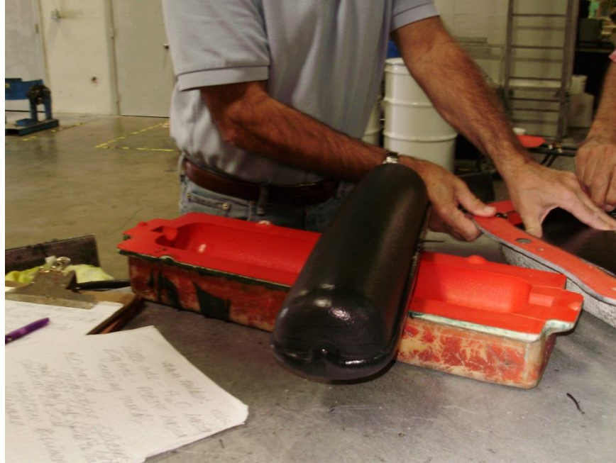
Figure 3-7 Long Part Made with Mold Release Agent at Fold Molders
