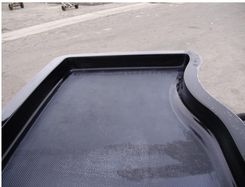
Figure 3-1 Non-Skid Area on Mold
