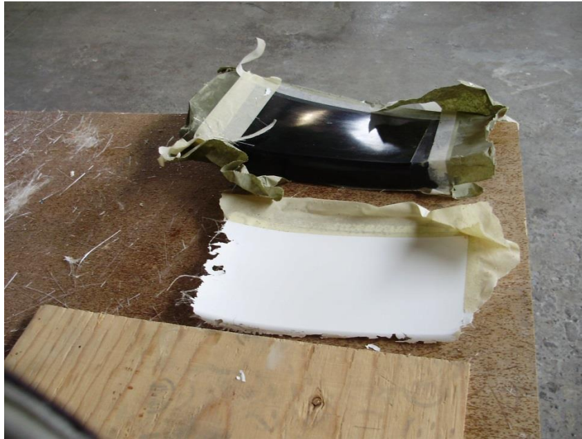
Figure 3-5 Parts Made with Water-Based Mold Release Agent at FinCo
